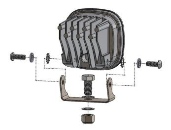
6. Close the hood. Now with the 9/16" wrench and socket, the lights can be placed onto the A-pillar brackets, aimed, and tightened.
