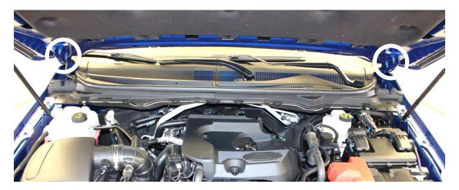
Place masking tape along the hood hinges (shown below) to ensure proper realignment. Also, place masking tape along the back edge of the hood near the windshield to prevent any scratches when aligning the bracket.
